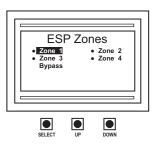
The factory default for all zones is active ESP function as indicated by the bullet  $(\bullet)$  next to each zone. To deselect a zone, press the UP or DOWN button until the bullet disappears.
