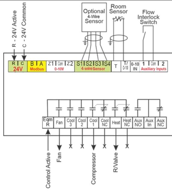
This is similar to a standard single stage heat pump except that the auxiliary input is set to shut the Saturn down on loss of water, thereby protecting the system.
