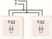
Examples of averaging in 2, 3 and 4 locations are shown using a combination of 2-wire sensors.
