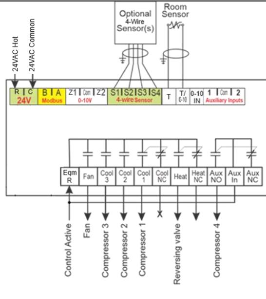
In this example the Saturn is running a heat pump system with 4 compressors providing 4 stages of heating and 4 stages of cooling.
