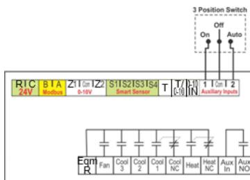
In the Auto position the Saturn will run its normal 7 day or 365-day schedule. In the ON position the Saturn will use the START program temperatures and fan mode for as long as this switch is closed. In the OFF position the Saturn will shut down.
