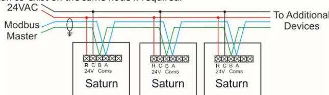
Some simple rules apply with Communications wiring; all devices **MUST** be in series No "T" branches or "star" wiring will be tolerated as this will seriously degrade or stop communications.
