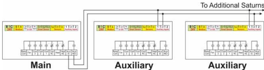
**Main –** Set Aux Relay Function to “Master” Mode in the installer menu. This will close the Aux Relay whenever the master Saturn is running. Should the Saturn receive a call to run outside scheduled hours.
