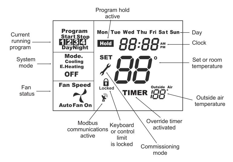
The T-32-P2 is capable of many advanced control options. Not all LCD symbols may appear on your specific thermostat configuration.
