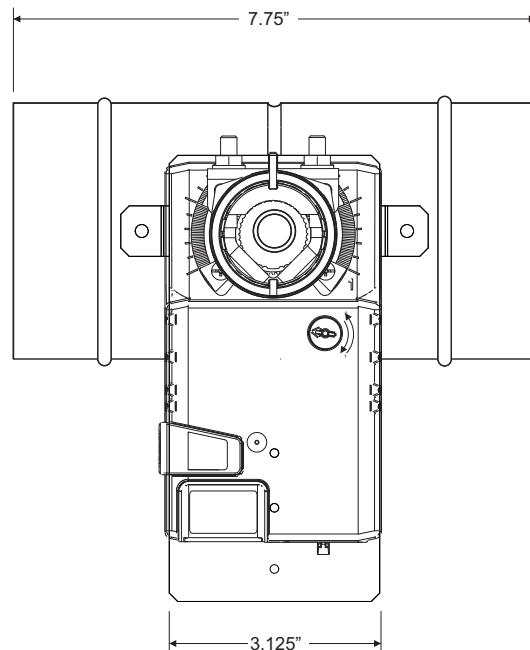
The OAD-XX-MOD is designed for retrofit or new construction applications requiring exhaust, fresh air intake, and zone control applications. Typical application use includes bathrooms/restrooms and individual rooms in high rise hotels, office buildings and apartment buildings. The damper is equipped with a 2-10 V (4-20 mA) modulating actuator.
