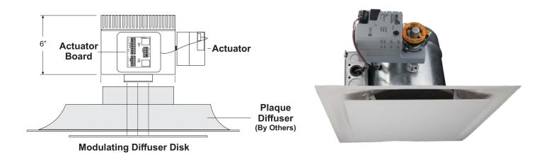
The iO HVAC Controls VD-RK is a complete modulating VAV diffuser retrofit kit designed to fit Nailor®, Carnes®, Krueger, Titus and many other 24" x 24" plaque diffusers with standard neck sizes of 6", 8", 10", 12" and 14".
