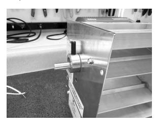
4. Install minimum position collar onto the damper shaft. Tighten down set screw in desired position.
