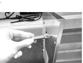
3. Install the CD-ZD-SD-EB shaft adapter and tighten down set screw.
