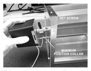
2. With the damper in the spring return open position, loosen the set screw for the shaft adapter. Remove actuator assembly. Set aside minimum position collar.
