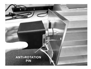
5. Align anti-rotation pin and install the HD-MOTOR-RR onto the damper shaft. With damper blade in open position, tighten down set screw.
